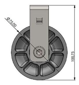
• Outer diameter: 75 mm • Total height: 100,75 mm
