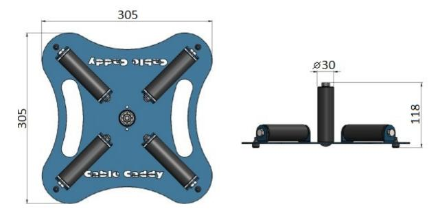
Thanks to its sophisticated design, the CableCaddy X has a secure footing - even when unwinding larger cable reels or pulling the cable a little harder Dimensions: 305 x 305 x 118 (mm)
