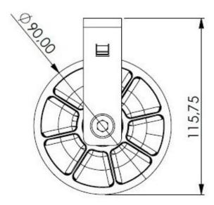
• Outer diameter: 90 mm • Total height: 115,75 mm
