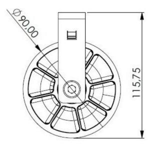
Outer diameter: 90 mmTotal height: 115,75 mm
