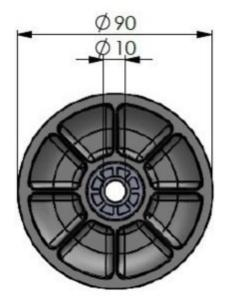
Outer diameter: 90 mmcompatible with 10 mm bolt
